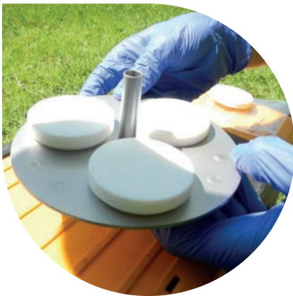
Chemcatcher® discs (photo courtesy of WRT)
